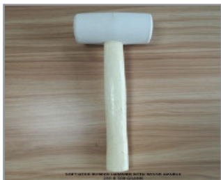
Figure 1 Mallet (Rubber Hammer -500gm)
