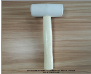
Figure 1 Mallet (Rubber Hammer -500gm)
