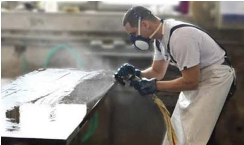
Fig:- (f) Smooth quartz edges using abrasives.
