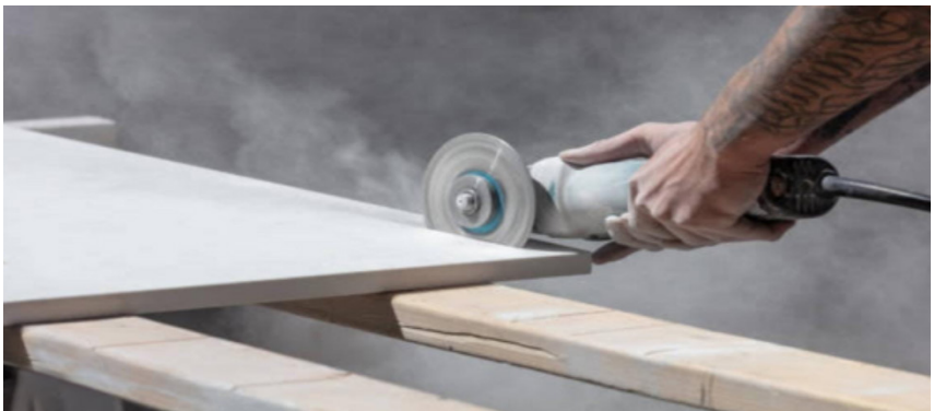
Fig:- (e) Cutting quartz slabs requires precision with diamond blade saws for clean, accurate results.
