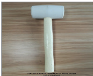
Figure 1 Mallet (Rubber Hammer -500gm)
